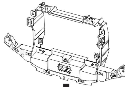
7. Remove hazard light switch from OEM panel.
